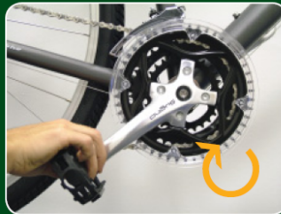
L. Right pedal finger tighten clockwise
