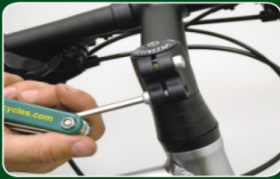
A. Slackening and tightening stem bolts
