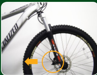
I. Position the fork so disc brake is at the rear
