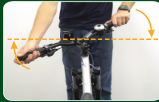
B. Twist stem into position
