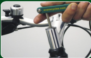
D. Slackening and tightening top bolt
