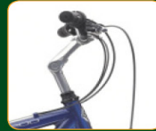
QUILL SYSTEM The stem is slotted into the fork steerer tube
