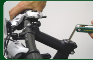
C. Tighten the top bolt
