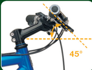
G. Position handlebars so the levers are 45° to the ground
